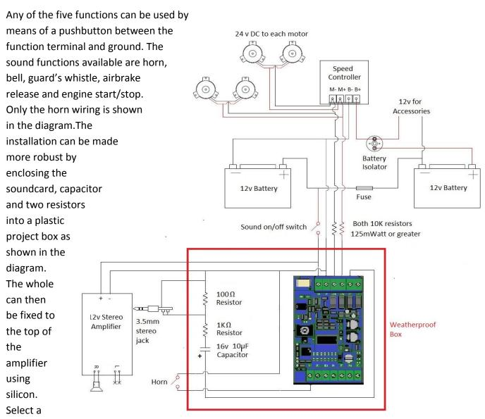
speaker which matches the impedance and power output of the amplifier. In the case of the Jaycar AA0487 a 15 watt speaker of four ohms impedance is needed. It is also important to make a soundbox which is an airtight fit to the back of the speaker. This will improve both volume and sound quality.
