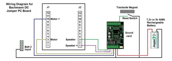
PP3 or a 7.2v cordless phone battery is used to drive the soundcard and produce sound when the loco is static or moving slowly. This battery will be automatically recharged whenever the motor voltage is at about 1.8 volts higher than the battery voltage so there should never be a need to remove the battery for recharging. However, the battery must be a Nickel Metal Hydride type; Lithium and Nickel Cadmium batteries must not be used.
