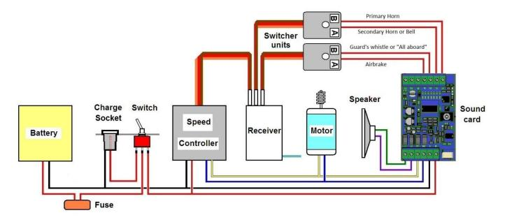
The receiver shown has two function channels, each of which can operate two triggers via two switcher units. The fifth soundcard trigger, the turbocharger, therefore cannot be radio controlled and will need to be switched on, if required, by the IR remote control. A suitable switcher unit is the Pololu 2802.
