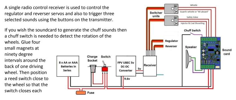
time a magnet passes. The soundcard will then chuff four times per wheel revolution.
