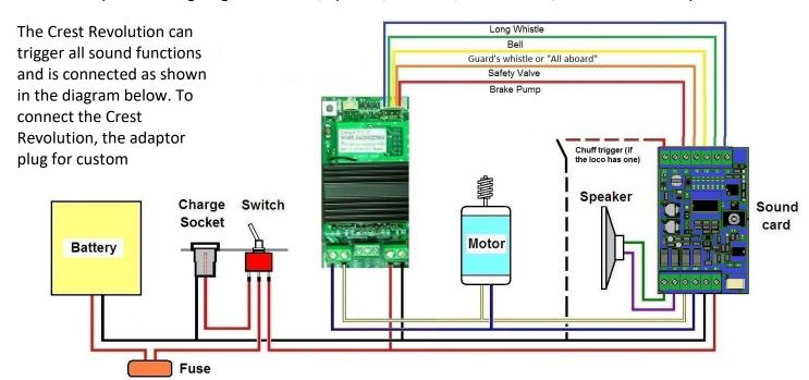
installations is used with the outer red, orange, grey and black wires being connected as shown. The whistle and despatch functions should be set to momentary by selecting MENU – ASSIGN FUNCTIONS – AUX FUNC SETUP.
