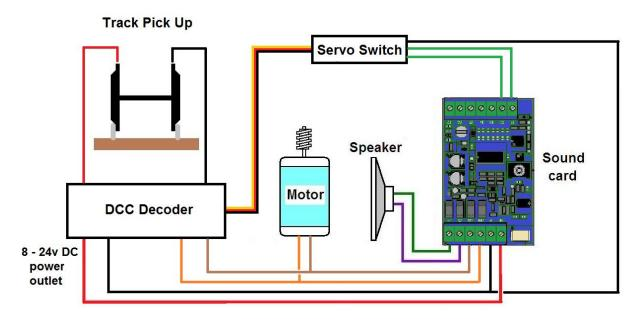
cannot trigger sounds directly from the controller. Therefore the above methods are used to trigger the sounds. Some decoders have a servo output which can be used to trigger sounds from the controller buttons by using a servo switch. They may also have a constant DC power output which can replace the battery if it is in the voltage range 8 to 24 volts. These connection options are shown below:
