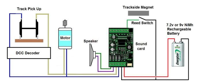
When the motor voltage is below seven volts it is insufficient to power the soundcard. Therefore a 9v volt PP3 or a 7.2v cordless phone battery is used to drive the soundcard and produce sound when the loco is
