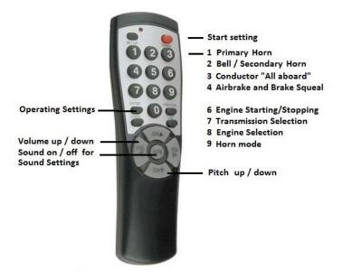
Note that the buttons on the remote control auto-repeat if held down. If you want a single event to occur, like turning on the safety valve, then press the safety valve and release it immediately. If you want to make a large change in volume or tone then you can hold the button down to avoid the need to press the button repeatedly.
