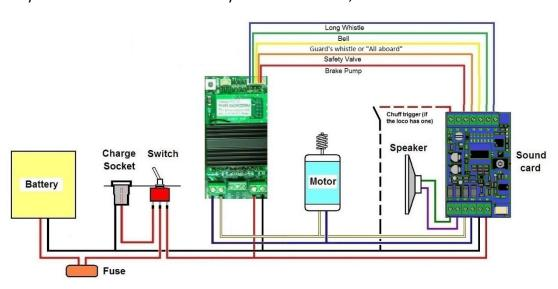
A chuff switch can be set up on the tender or van wheels. The soundcard automatic modes can be used to make a whistle sound on departure and at timed intervals. Other sounds can also occur automatically using the modes provided. A rechargeable PP3 battery should sustain continuous running with an automatic whistle for about two hours.
