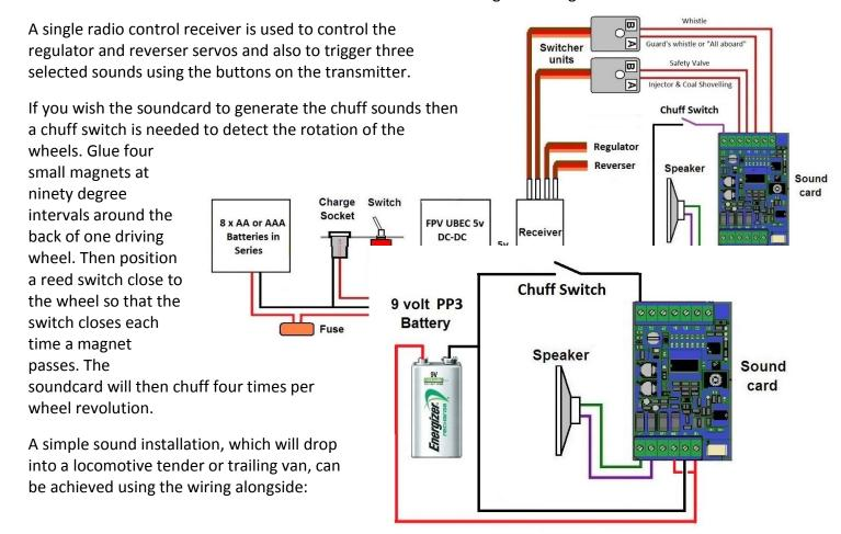
A chuff switch can be set up on the tender or van wheels. The soundcard automatic modes can be used to make a whistle sound on departure and at timed intervals. Other sounds can also occur automatically using the modes provided. A rechargeable PP3 battery should sustain continuous running with an automatic whistle for about two hours.
