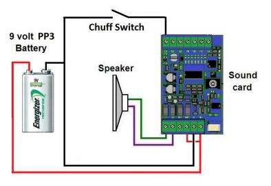
The most common way of doing a chuff switch is to use a reed switch positioned close to the back of a tender or van wheel and then glue magnets around the back of the wheel as follows:
