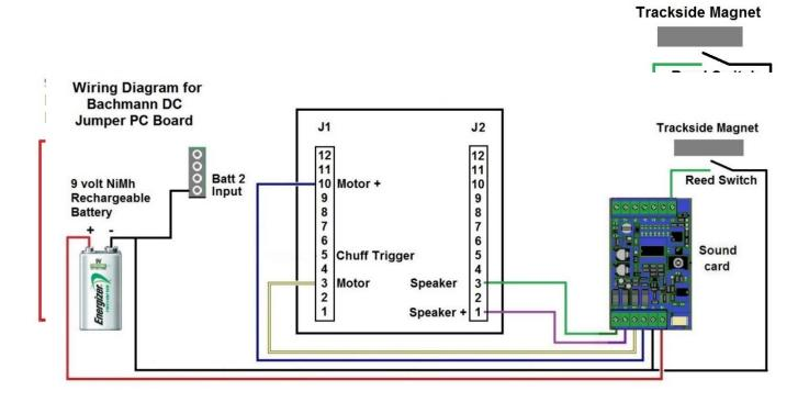
The wiring diagram below shows the connections for the DC jumper board in a Bachmann locomotive.
