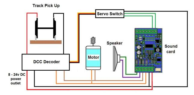
cannot trigger sounds directly from the controller. Therefore the above methods are used to trigger the sounds. Some decoders have a servo output which can be used to trigger sounds from the controller buttons by using a servo switch. They may also have a constant DC power output which can replace the battery if it is in the voltage range 8 to 24 volts. These connection options are shown below:
