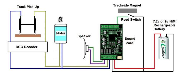
When the motor voltage is below seven volts it is insufficient to power the soundcard. Therefore a 9v volt PP3 or a 7.2v cordless phone battery is used to drive the soundcard and produce sound when the loco is
