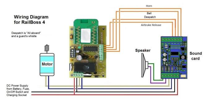
The RailBoss 4 can trigger four sound functions. The fifth and sixth soundcard triggers, the turbocharger and engine start/stop, therefore cannot be radio controlled and will need to be switched on, if required, by the IR remote control or be set to sound automatically.
