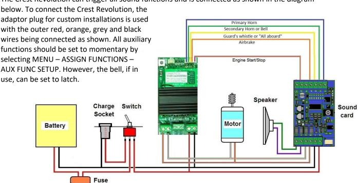
Note also that early Revolution receivers, without the onboard sound, will start the soundcard immediately when power is switched on. However this will not happen with later Revolution receivers with the onboard sound. With the later ones you will need to throttle up three button presses to switch on the sound which will then stay on.
