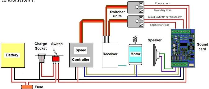
The receiver shown has two function channels, each of which can operate two triggers via two switcher units. The fifth soundcard trigger, the turbocharger, therefore cannot be radio controlled
