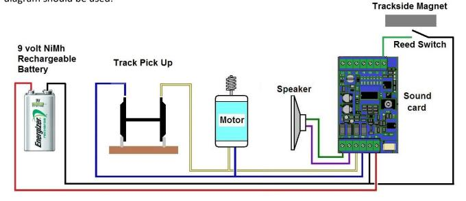
The wiring diagram below shows the connections for the DC jumper board in a Bachmann vehicle.
