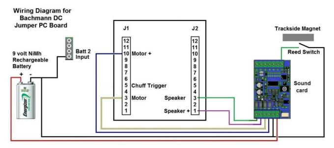
On DCC track powered railways in locomotives using a basic decoder, the wiring is a little different:
