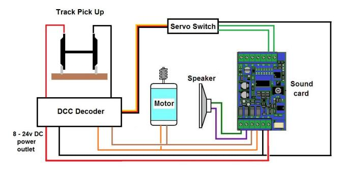
can be used to trigger sounds from the controller buttons by using a servo switch. They may also have a constant DC power output which can replace the battery if it is in the voltage range 8 to 24 volts. These connection options are shown below:
