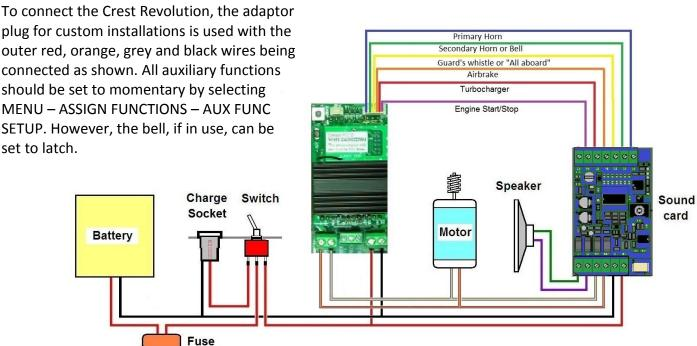
Note also that early Revolution receivers, without the onboard sound, will start the soundcard immediately when power is switched on. However this will not happen with later Revolution receivers with the onboard sound. With the later ones you will need to throttle up three button presses to switch on the sound which will then stay on.
