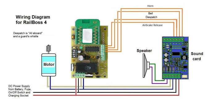
The RailBoss 4 can trigger four sound functions. The fifth and sixth soundcard triggers, the turbocharger and engine start/stop, therefore cannot be radio controlled and will need to be switched on, if required, by the IR remote control or be set to sound automatically.
