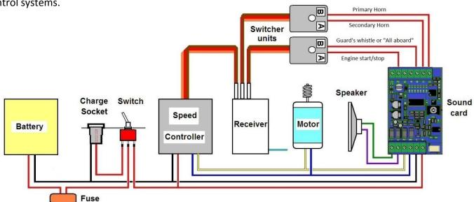
The receiver shown has two function channels, each of which can operate two triggers via two switcher units. The fifth soundcard trigger, the turbocharger, therefore cannot be radio controlled and will need to be switched on, if required, by the IR remote control. A suitable switcher unit is the Pololu 2804.
