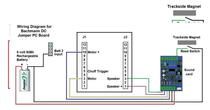
The wiring diagram below shows the connections for the DC jumper board in a Bachmann locomotive.
