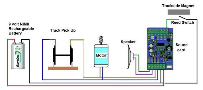
The wiring diagram below shows the connections for the DC jumper board in a Bachmann locomotive.
