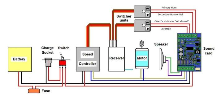
The receiver shown has two function channels, each of which can operate two triggers via two switcher units. The fifth soundcard trigger, the turbocharger, therefore cannot be radio controlled and will need to be switched on, if required, by the IR remote control. A suitable switcher unit is the Pololu 2804.
