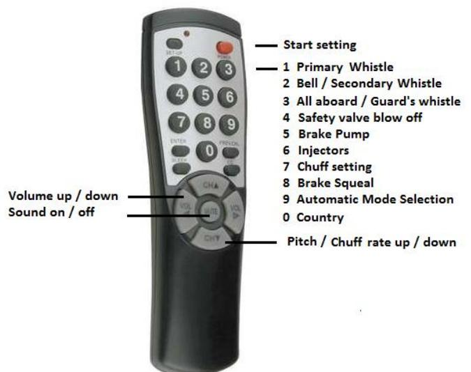
Note that the buttons on the MyLocoSound remote control auto-repeat if held down. If you want a single event to occur, like turning on the safety valve, then press the safety valve and release it immediately. If you want to make a large change in volume or tone then you can hold the button down to avoid the need to press the button repeatedly.
